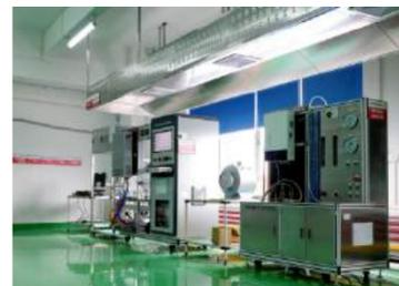
Water Heater Integrated Automatic Testing Equipment
